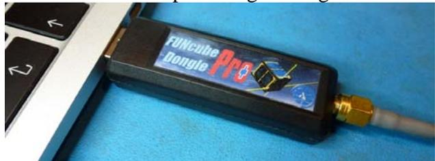
The FUNcube Dongle is a software defined radio (SDR) that fits into a 'USB key' and is part of AMSAT-UK's FUNcube satellite project. The FUNcube Dongle allows anyone to try their hand at reception of satellites like the FUNcube, due for launch in November 2012, as part of a global educational collaboration project collecting information from space.
